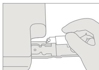
2 Place microcuvette into photometer.
