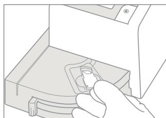
2 Place microcuvette into analyzer.
