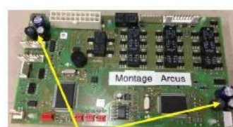
Board with dual components in case of failures
